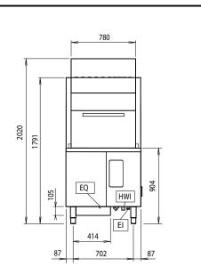
Drain Electrical inlet (power) FΩ **Electrical Outlet** HWI Hot water inlet Detergent connection
